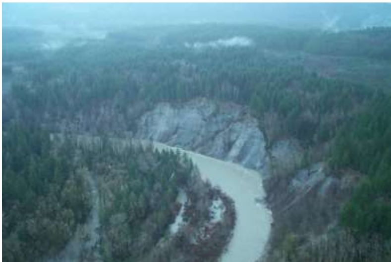
Photo 1. Aerial upstream view of the Stoltz slide that releases fine clay sediments and extends for 600 m along the left bank for the mainstem Cowichan River. Remedial works undertaken in 2006 and 2007 have successfully reduced bank erosion and sedimentation (Sheng and Bonnell 2010).
